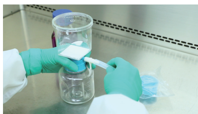
2. Ensure the handle is positioned vertically downward, then connect the vacuum pump tubing to hose connector.
