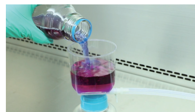
3. Open the cup lid and add the solution to the funnel.
